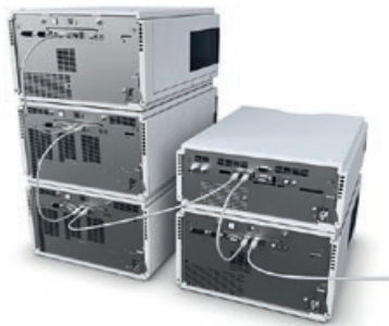
Figure 3.49 CAN communication lines – fast direct communication between the modules is independent from the host software.
