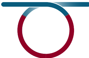
Figure 3.9 Partial fill of sample loop.
