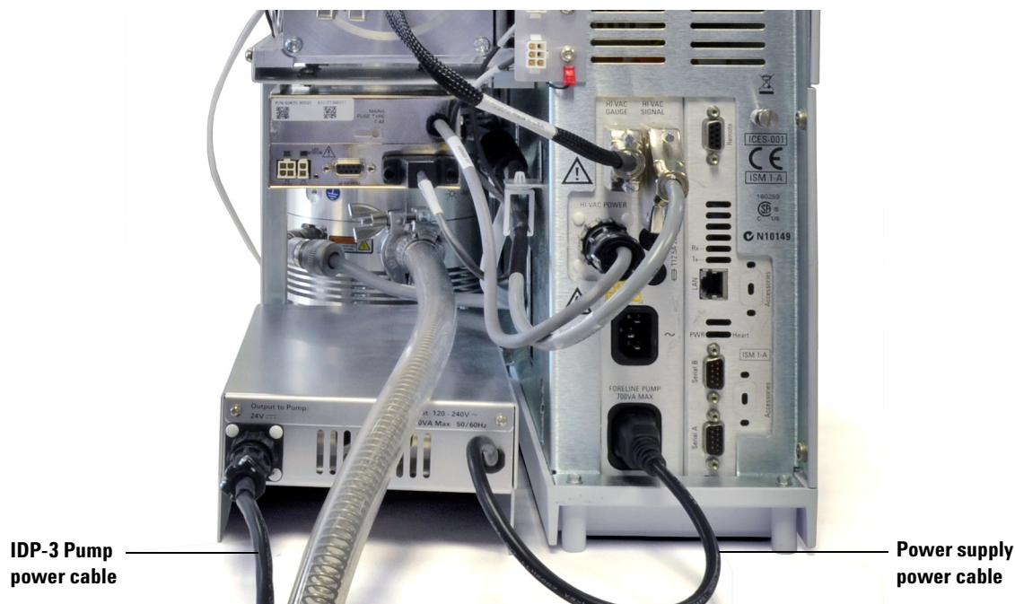
Figure 15 IDP-3 power supply cabling
