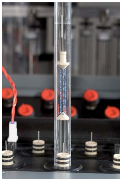
400-DS sample cell with stent holder
