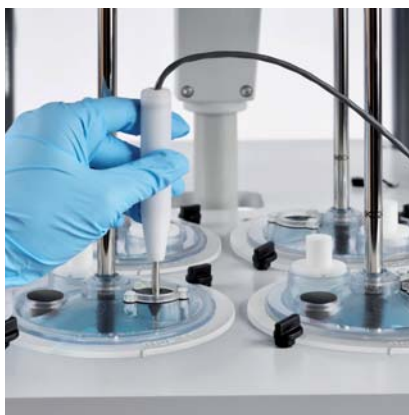
Manual temperature measurement using 708-DS temperature probe
