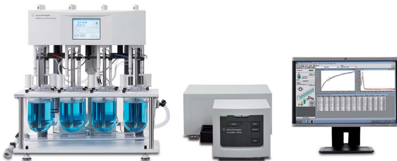
The 708-DS, 850-DS with the Cary 8454 provide an online UV system controlled by ChemStation UV-Vis Software
