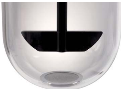
USP Apparatus 5 Paddle Over Disk
