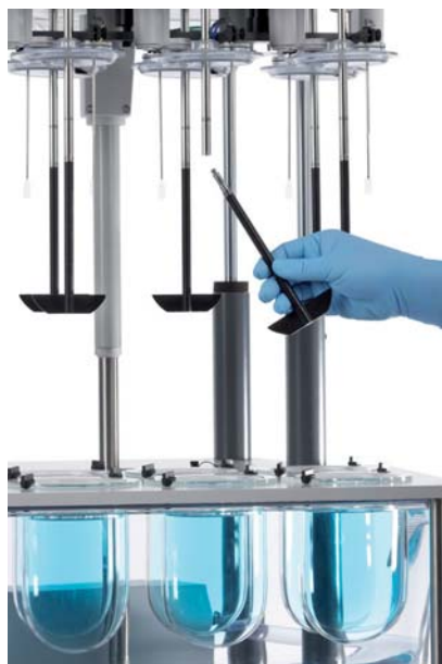
Upper shaft receptor and lower paddle piece
