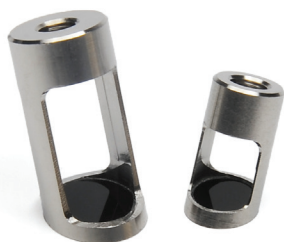
Fluorescence fiber optic liquid tips kit, 9910104500
