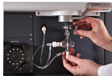
Multimode Sample Introduction System (MSIS)
