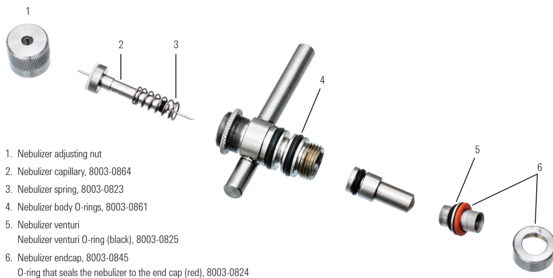
Exploded view of Nebulizer assembly, 8003-0828
